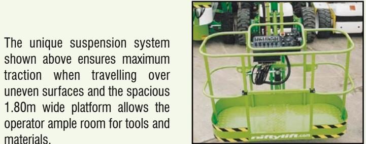
The unique suspension system shown above ensures maximum traction when travelling over uneven surfaces and the spacious 1.80m wide platform allows the operator ample room for tools and materials.
